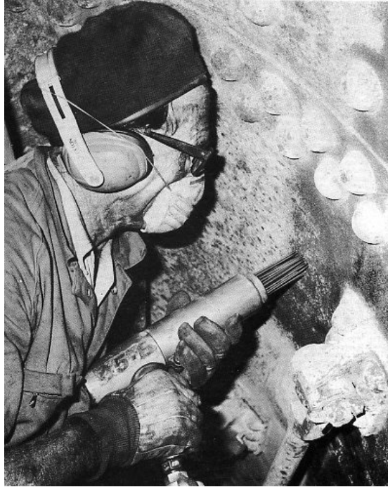
Needlegunning inside 621's boiler. Never a popular job but Howard Johnston has spent many hours removing layers of scale Photo: Roger Currie
