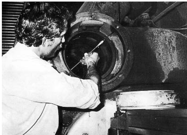
Ian Johnston checks measurements of the rebored valve cylinders. Note one of the four new bull ring castings on slide bars. Photo: Roger Currie
