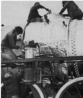
Peter Hoye and Peter Soar tightening dome cover nuts as Glen Smythe and Andrew Gramp work on insulation cladding (L) and Richard Bonney and Roger Currie fit insulation to 621's cylinders (R)
