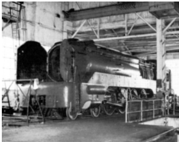
520 as Islington undergoing a boiler inspection
