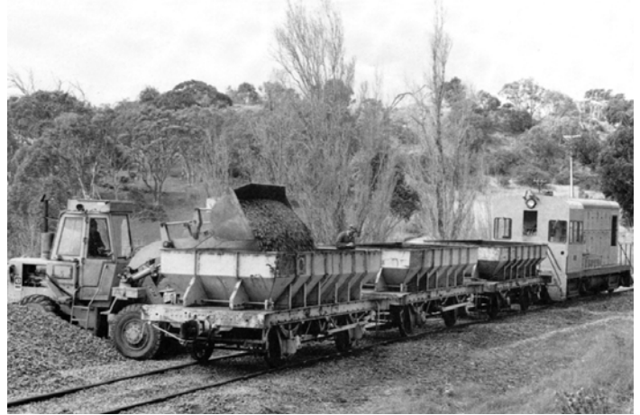
Ater running one train load of ballast DE351 pauses at Gemmels so that three of the SteamRanger Z class hopper wagons can be reloaded Photo: Roger Currie
