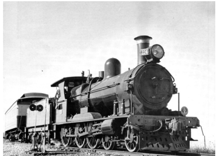
Rx224 leaving Goolwa Depot with the Cackle Train for its first run of the day on 4 January 1988. Note the two switchstands, one of which is provided to bolt lock the switch for the main line. Goolwa Depot is situated 2km from Goolwa and this arrangement enables trains to negotiate the facing switch at speed when not calling at the depot. Photo: Roger Currie
